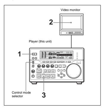
1 Power on this unit by pressing the  $\circlearrowleft$  switch on front panel.
